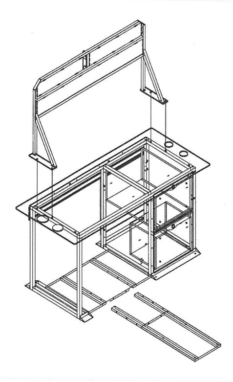
When installing the overhead unit, take (4) of the  $\frac{1}{2}$ -20 x 2" bolts and nuts found packed in the gaylord box with overhead unit.
